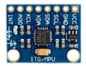
Figure2.2. MPU6050 IMU
