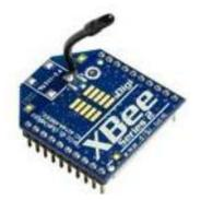
Figure 3. Xbee S2C radio transceiver
