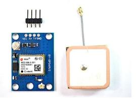
Figure2.4 NEO 6M GPS Module
