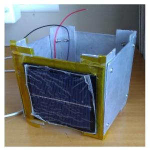
Figure 5.5 Aluminum CubeSat structure
