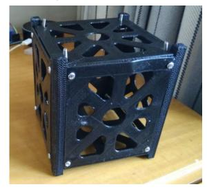
Figure 5.4 3D printed CubeSat structure
