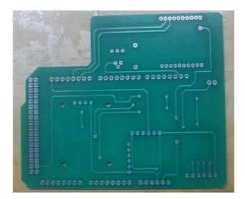
Figure 7.4 Final PCB for the glider sat(Back)
