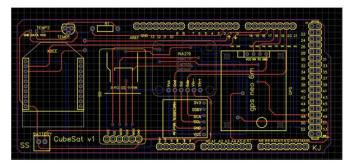
Figure 7.1 Initial PCB design for the glider sat
