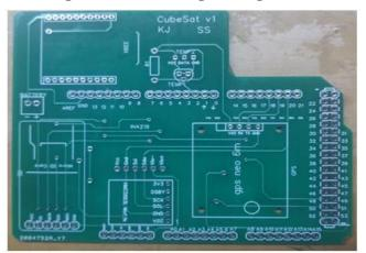
Figure 7.3 Final PCB for the glider sat(Front)
