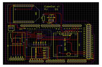
Figure 7.2 Final PCB design for the glider sat
